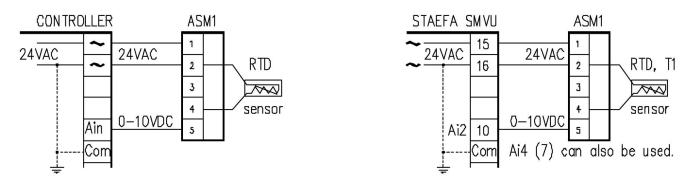
The ASM1/RTD-1K/10V/0-100/S or ASM1/T1/10V/0-100/S interface module is factory set up to receive a 0-100°F resistance signal from a RTD or STAEFA's T1 temperature sensor and provide a voltage output inputs. The stand-alone version provides an internal pull-up resistor, while the parallel version has a high input impedance as to not load the existing sensor circuit.
