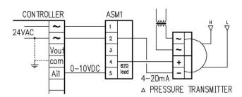
The ASM1/mA/VDC/P (potted version) is factory configured to accept the 4-20mA signal from a 4 wire transmitter. The 4-20mA signal is fed into a 62 Ohm load resistor, referenced to common, and provides an adjustable voltage output from 0-3V to 0-10VDC.
