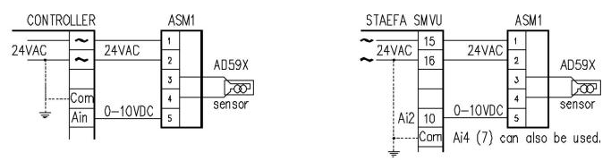
The ASM1/AD59X/10V/0-100/P interface module is factory set up to provide a +15VDC power source for an AD590 or AD592 temperature sensor and receive a 0-100°F signal and provide a 0-10VDC output. The ASM1 output is scaled for a specific temperature range allowing other sensors to be used with controllers that have a specific sensor type input.
